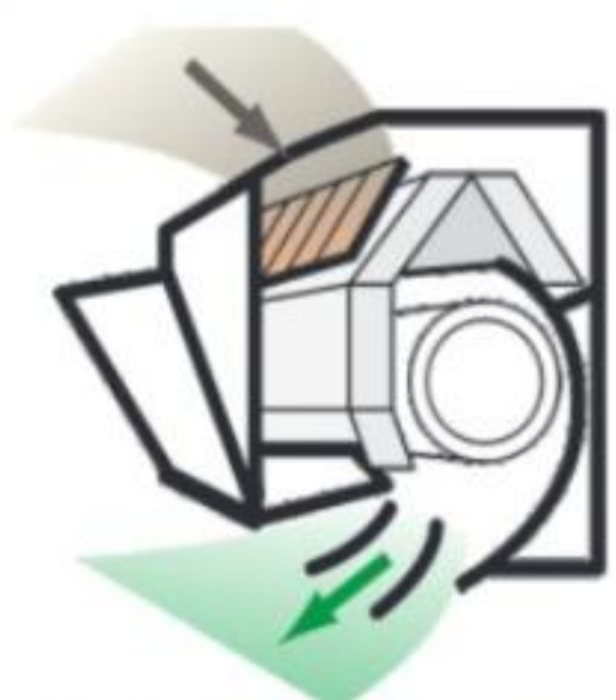
Catching Allergen on the Filter
